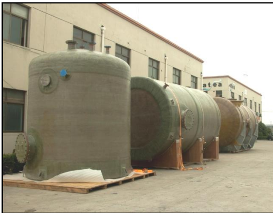
Two examples of our recently produced large tanks for use in hazardous chemical storage applications
